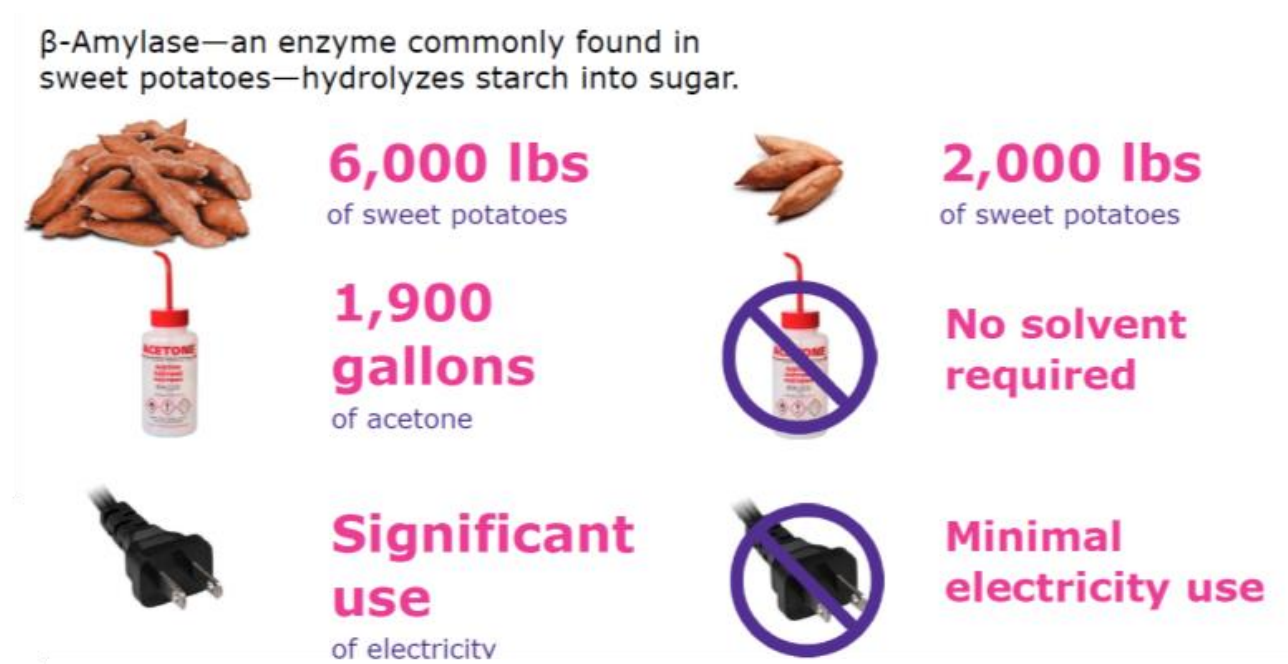
Figure 7. Impacts of re-engineering \beta -Amylase process.
